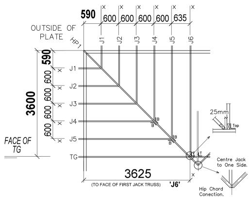
Fix Jack Trusses (J4,J5,J6 Etc) with 1/Triple Grip to Hip Truss and Truncated Girder Truss.
